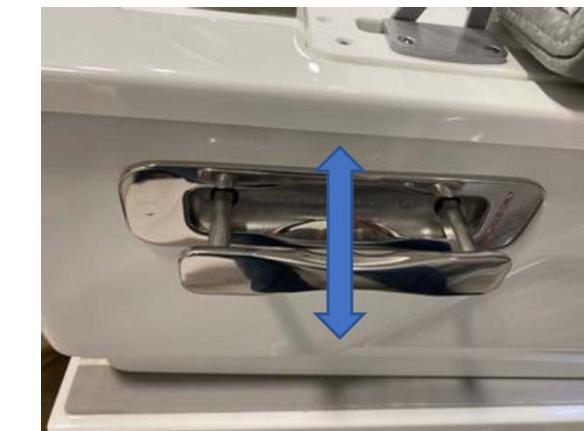
Are pull-out devices like the above shown deemed to be handholds if installed according to the location and strength requirements as per chapter 9 of EN ISO 15085?
