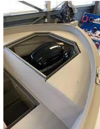
A lot of the time the petrol tank and filter connections are also placed in this same engine closed well, the closed well will thus house the petrol tank, outboard engine and all relevant assembly fittings including filters and hoses. Such an installation thus has all the characteristics of a petrol inboard engine as the compartment is closed during sailing.
