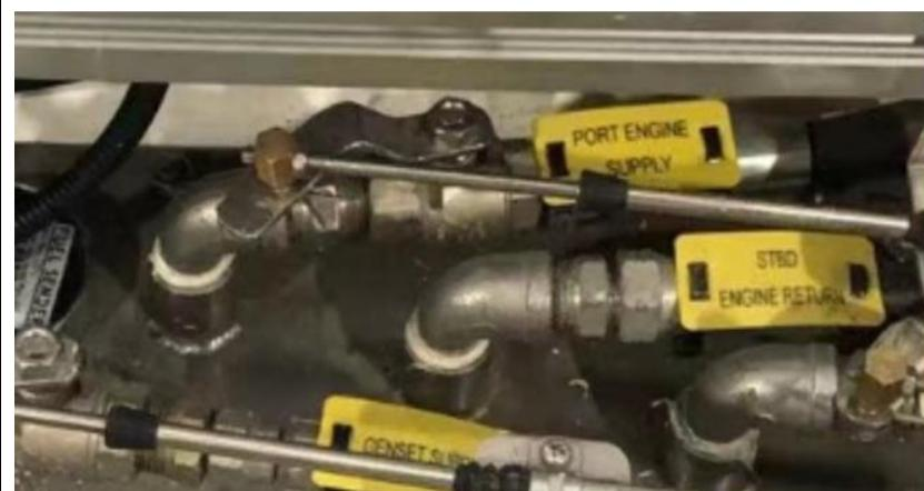
(Note: if the answer is no, the elbow is a separate fitting between tank and valve. This would mean that all elbows would have to be welded to the tank's spigot, to make it a part of the tank. The tank's manufacturer may have supplied the tank off the shelf after a pressure test and further welding by the boat manufacturer introduces unnecessary risk and invalidates the warranty).
